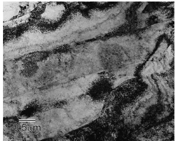
Fig. 5. Transmission electron micrograph of 12YWT after creep for \approx 14\,500 h at 800 °C and 138 MPa.
